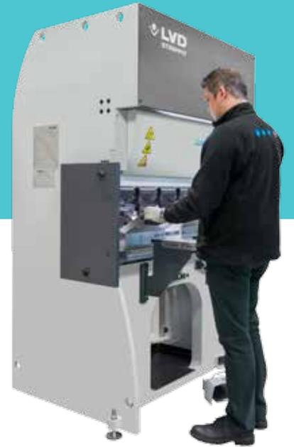
The *Dyna-Press* standard models 12/8 and 24/12 are equipped with a back gauge with **2 axes** (X,R). The *Dyna-Press* 24/12 Plus model has a back gauge with **4 axes** (X,R,Z1,Z2).
