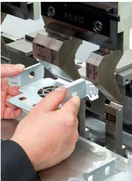
The **electric drive** Dyna-Press series are now available with 12 and 24 tons of bending force and a working length of 33" and 49".
